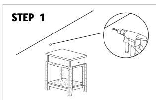
1. Find spot on wall 1" below top of item. 2. Using a drill bit slightly thinner than anchor, drill hole into drywall.
