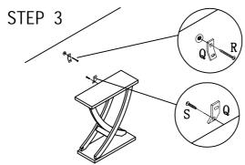
1. Insert drywall screw into metal bracket and into drywall anchor. 2. Insert flathead screw into second metal
