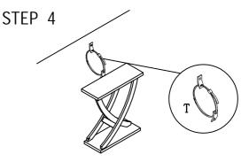
1. Insert strap thru bracket attached to wall. then thru bracket on item, and into head of strap. 2. pull lightly til strap stops. Assembly is complete.
