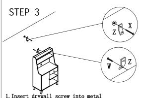
bracket and into drywall anchor.
