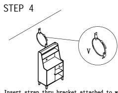
1. Insert strap thru bracket attached to wall. then thru bracket on item, and into head of strap. 2. pull lightly til strap stops.
