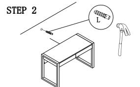
1. Use a light hammer to tap anchor into hole.
