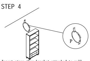
1. Insert strap thru bracket attached to wall. then thru bracket on item, and into head of strap.
