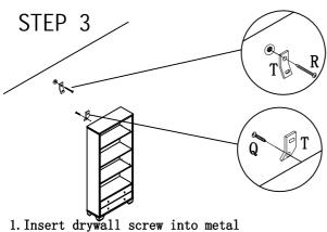
bracket and into drywall anchor.
