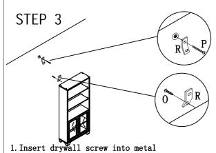
bracket and into drywall anchor.
