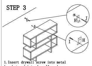
bracket and into drywall anchor. 2. Insert flathead screw into second metal bracket and into back of item. along top edge.
