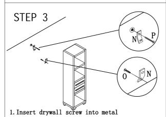
bracket and into drywall anchor.
