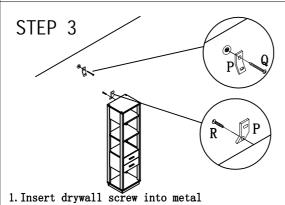
bracket and into drywall anchor.
