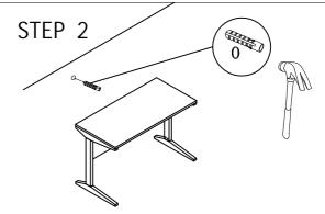
1. Use a light hammer to tap anchor into hole.
